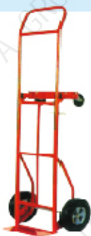
HT1921 Weight(kg):18.2 Load Capacity(kg):200 Solid Tyre:10"x2.5" L/W/H(mm):1688x505x418
